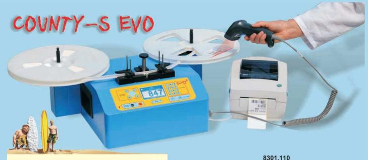
COUNTY-S EVO is a motorized counting machine for taped SMD component counting.
