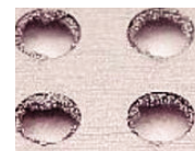
Partially blocked apertures
