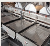
IsoThermal Convection Preheat (ICP)
